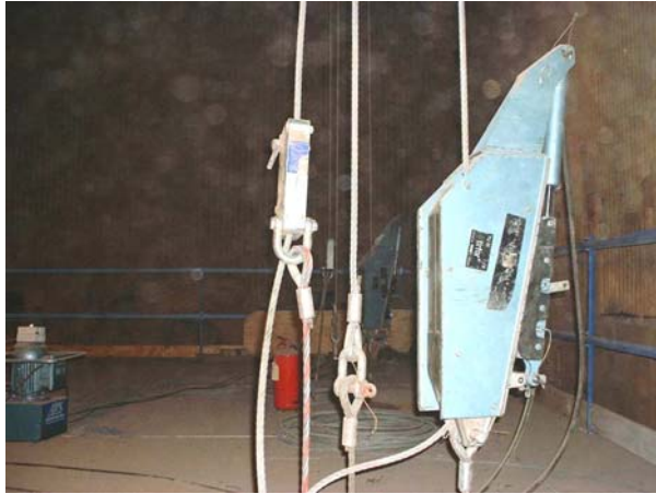
^ 3200Kg Hoist and secondary safety devise
