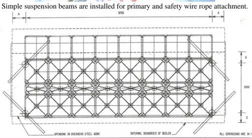
For this application overall platform dimensions are 9.76M X 3.00M (4.30M with hinged section down)
