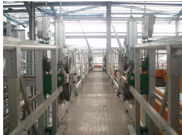
Hand operated hoists and safety devices raise and lower the platform, manual wire rope coilers store the wire ropes on board
