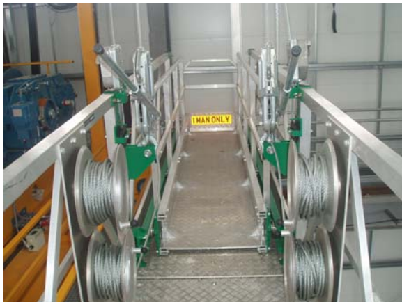
Hand operated hoists and safety devices raise and lower the platform, manual wire rope coilers store the wire ropes on board
